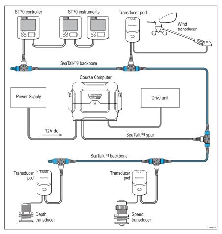
Note: SeaTalk<sup>ng</sup> system structures and load limitations: There are restrictions on cable lengths, power location and the number of components you may connect to a SeaTalk<sup>ng</sup> system. For complete information on SeaTalk<sup>ng</sup> connectivity, refer to the SeaTalk<sup>ng</sup> Installation Guide supplied with the SeaTalk<sup>ng</sup> Backbone Kit.
