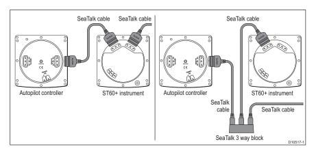
**Note:** If the controller is to be the primary controller, we recommend a direct connection to the system rather than daisy-chaining the controller to an instrument bus.
