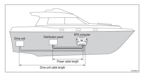
CAUTION: Use of incorrect power cable size could cause your SmartPilot to malfunction and will reduce the power supplied to the drive unit. Ensure the correct size is used and, if in doubt, use a heavier gauge cable.
