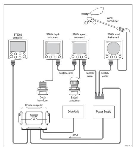
A SeaTalk based network does not have a central backbone cable. Connector blocks are used to connect different parts of the system.
