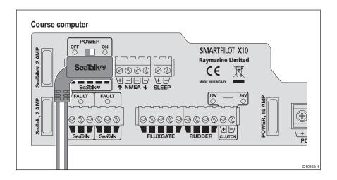
Connect the other end of the SeaTalk<sup>ng</sup> cable into a T-piece connector on the SeaTalk<sup>ng</sup> backbone cable or to a 3- or 5-way connector block.
